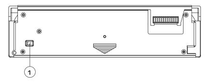
EJECT BUTTON: Press it to eject the disc from compartment.
